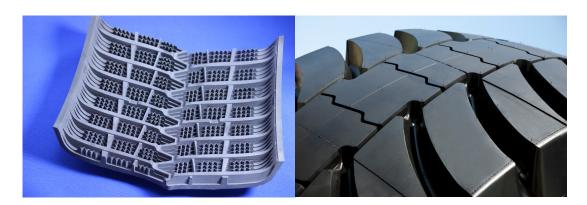
Caption: A section of tread mold created for the tire industry using high-strength managing steel 1.2709, printed on a 3D Systems ProX 300 3D Printer. Image courtesy of 3D Systems.
