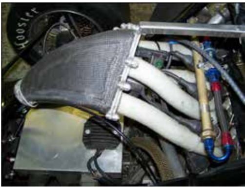
The evolution of the team's intake system (above): The top photo is a 1.3 L plenum with curved, tapered runners. Below that image is a 1.5 L plenum with curved runners built in a thicker material. Because of the curved runner, the injector is aimed at the back of the intake valve, allowing for more consistent vaporization. On the car (right) is a 1.4 L plenum with s-curve runners, allowing for a box formation in the plenum.
