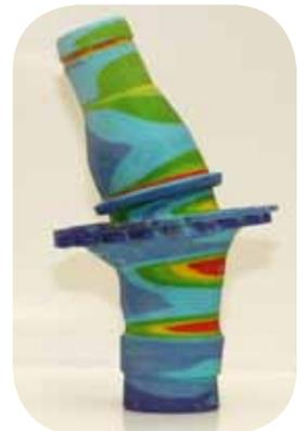
With the success of this innovation, Pratt & Miller engineers decided to test how well ZPrints worked for mold designs, and were pleasantly surprised with the results. They discovered they could use the ZPrinter to create wax infiltration molds for carbon fiber part production. And as it turns out, the molds not only work remarkably well with wax infiltration to produce accurate parts with smooth surfaces, but they can be used for multiple runs.
