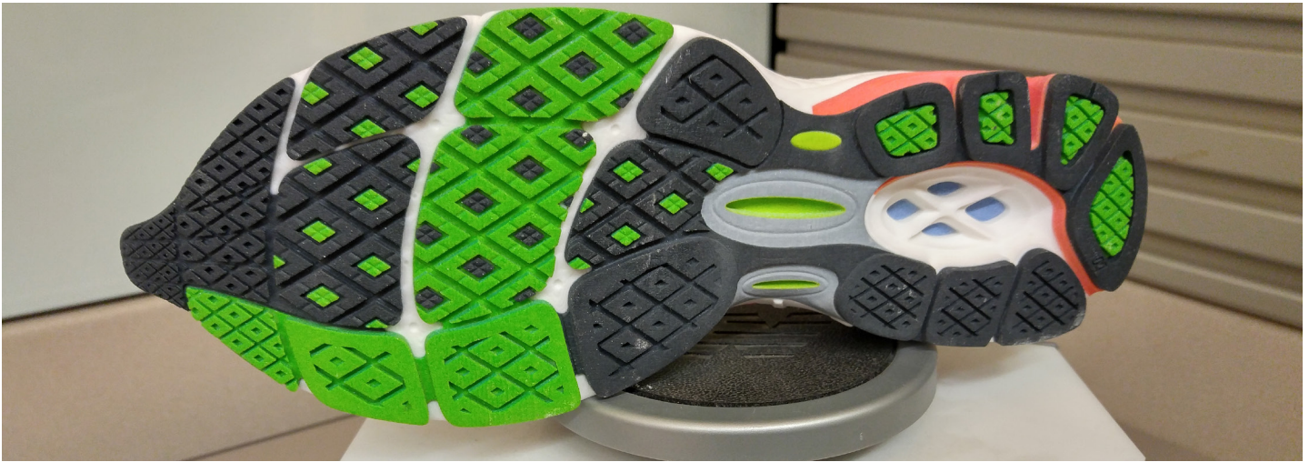
A 3D Systems ColorJet print of the New Balance 1260 V2 model shoe, showing design details and the range of colors available to visualize data with realistic prototypes.
