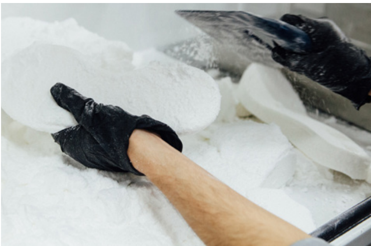
New Balance uses 3D Systems sPro SLS printers to produce prototypes in DuraForm Flex TPU material that provides the same properties as the foam used in manufactured shoes.
