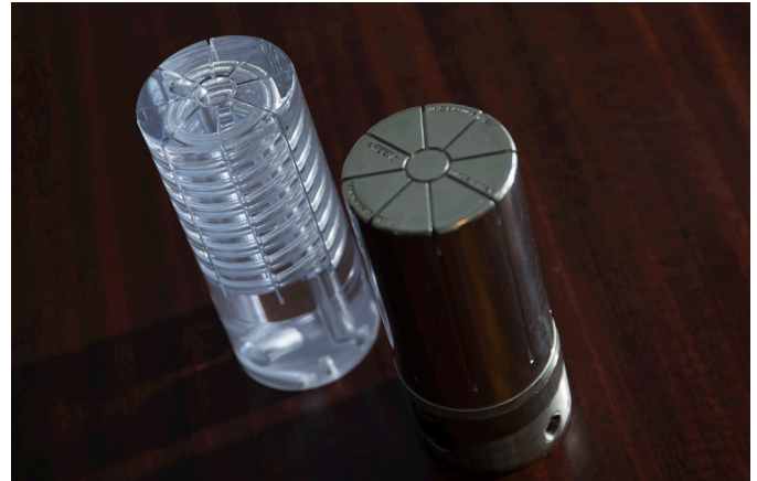
A Bastech mold core insert with conformal cooling channels prototyped using 3D Systems' Stereolithography (SLA) technology and printed in maraging steel on the ProX® DMP 200.
