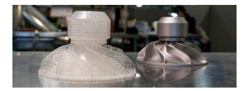
Traditional investment casting—creating metal parts from a ceramic mold after a wax pattern has been burned away—has been around for more than 5,000 years. Over the last century, the process has benefited from many innovations, but it is still slow and costly to create this kind of tooling for complex parts. Production time is typically measured in months and costs can run into the hundreds of thousands of dollars.
