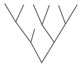
In this design you are diverging and so new entities are made instead of connected, thereby eliminating shrink lines.
