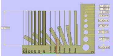
The smallest wall build up to a certain height, because than it starts to bend, because it is to fragile, this shows that we can perfectly build those walls but only for a limited height.
