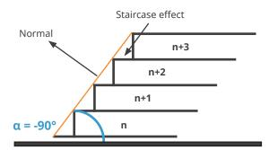
Upfacing surfaces are characterized by the normal of the object pointing away from the build platform
