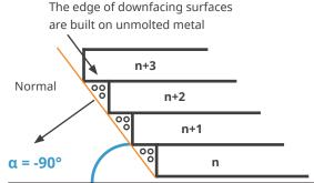
Downfacing surfaces are characterised by the normal of the object pointing towards the build platform.
