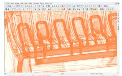
Mold with conformal cooling printed on a CNCed section of the mold
