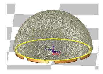
The inside of this part is hollow, so it contains a lot of powder. Holes at the bottom below the wire EDM offset to remove the powder
