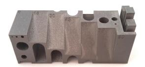
Example of **upfacing surfaces** in different angles ranging from: 0° (left) to 90° (right) with steps of 15°
