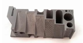
Example of **downfacing surfaces** in different angles ranging from: 75° (left) to 0° (right) with steps of 15°
