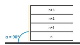
$\alpha$  = angle between horizontal build platform and tangent line of the object surface
