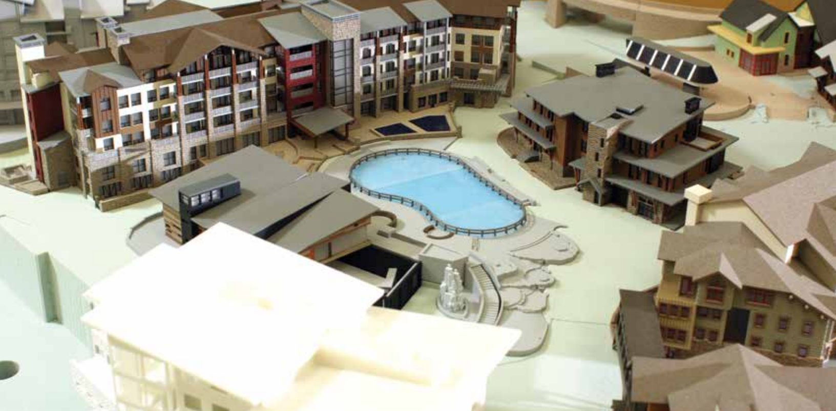
In total, approximately 250 individual pieces were printed to account for all the building shells, exteriors and landscaping features.
