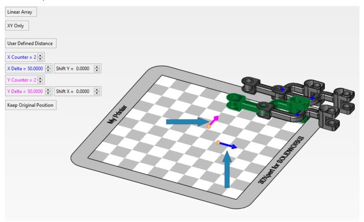
5. **Pick** the head of the two arrows (Pink and Blue) on the screen as seen in the picture above. This will Chang the direction of the copy instead of input – in the X & Y Delta:
