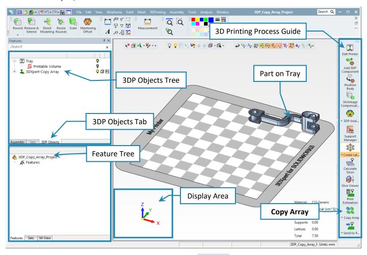
3. From the 3D Printing Process Guide access Copy Array
