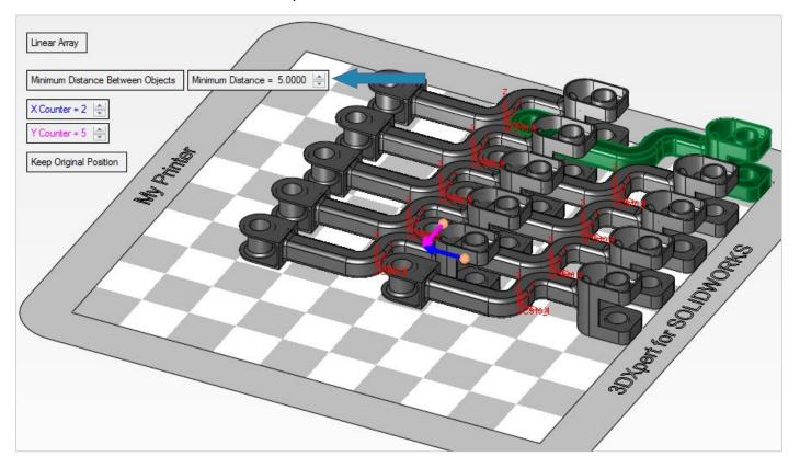
Note that in this mode of **Minimum Distance** the X&Y Delta are not displayed and that the systems ensues that the parts do not touch each other.
