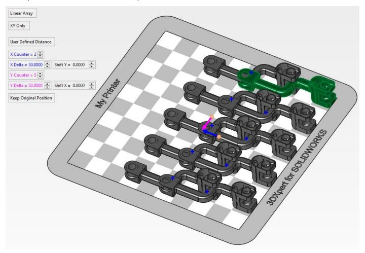
7. It is possible to copy array on **XY only** or also on Z direction. Change the parameter XY Only to **XY & Z** In this case, a 3D array is created in the X, Y and also Z direction.
