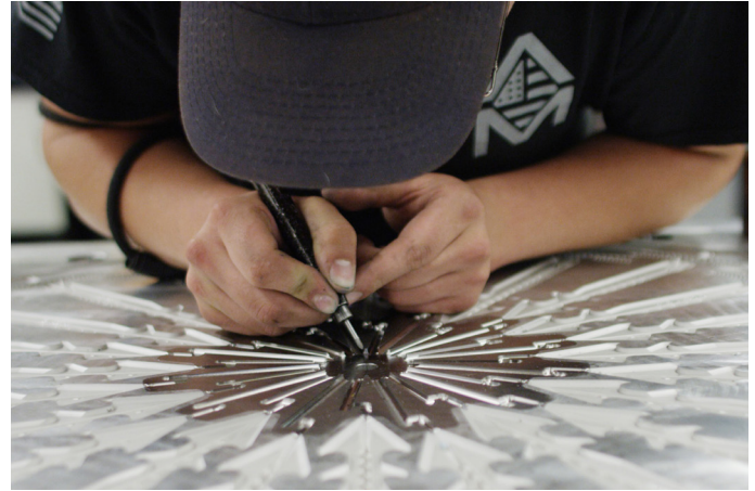
Polishing plastic injection mold designed and manufactured using Cimatron
