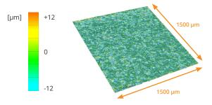
$\pmb{Smooth\ surface}$  as measured by a Keyence microscope, with an Ra down to 5.7  $\mu m.$
