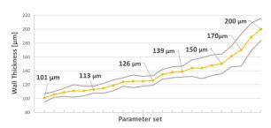
Extensive parameter database for  $\boldsymbol{customizable\ wall\ thickness}$  reliable down to 100  $\mu m.^2$
