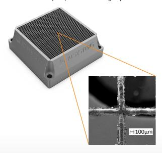
$<sup>^{\</sup>mbox{\scriptsize 1}}$  Surface treatment performed with zirconia blasting medium at 2 bar.
